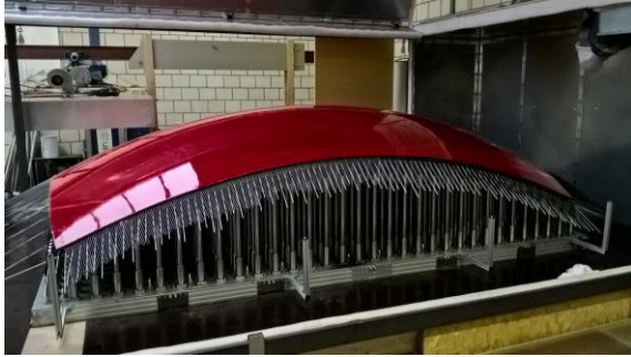
Figure 10: The adaptive mould at Curve Works
