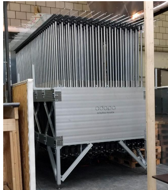
Figure 12: Demonstrating the actuator deflection of the Curve Works mould
