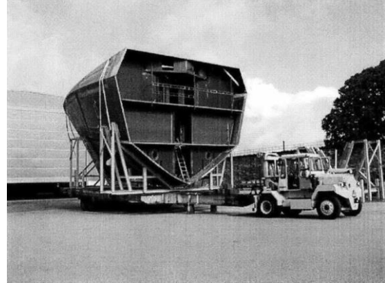
Figure 8: Bow section of the Visby-class corvette [6]
