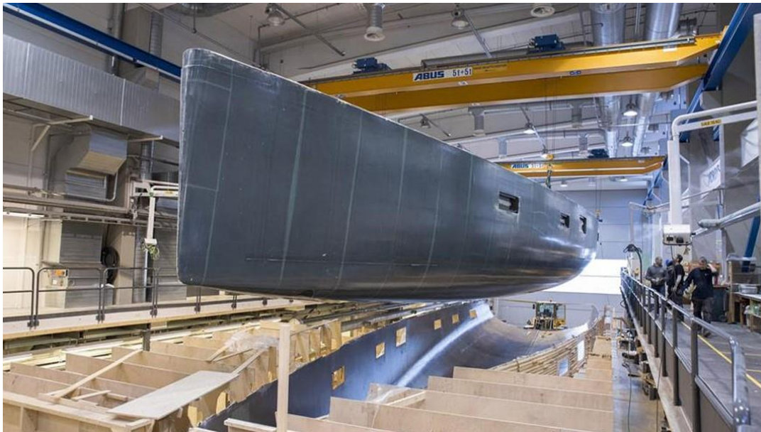
Figure 2: Demoulding the hull of the 34M superyacht (MM341) at Baltic. Courtesy Malcolm Mckean Yacht Design.
