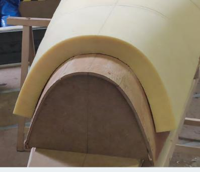
Above: a thermoformed single layer of 40mm Corecell™ M130 for the bow area of a super yacht
