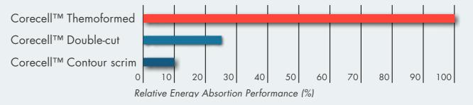
Comparison of energy absorption performance between thermoformed, scored & cut core. Dynamic testing by University of Auckland Centre for Advanced Composite Materials<sup>3</sup> confirmed that thermoformed core can absorb the same level of dynamic energy as virgin material.
