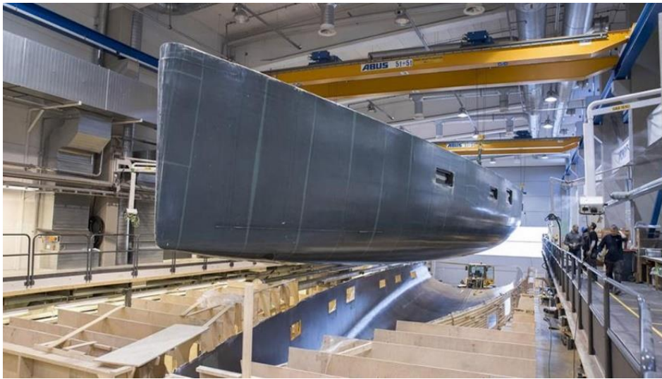
Figure 1: Demoulding the hull of the 34M superyacht (MM341) at Baltic Yachts. Courtesy of Baltic Yachts.
