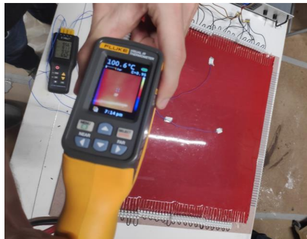
Figure 5: Functionality test of a membrane with integrated heating for a small adaptive mould showing uniform heat distribution.
